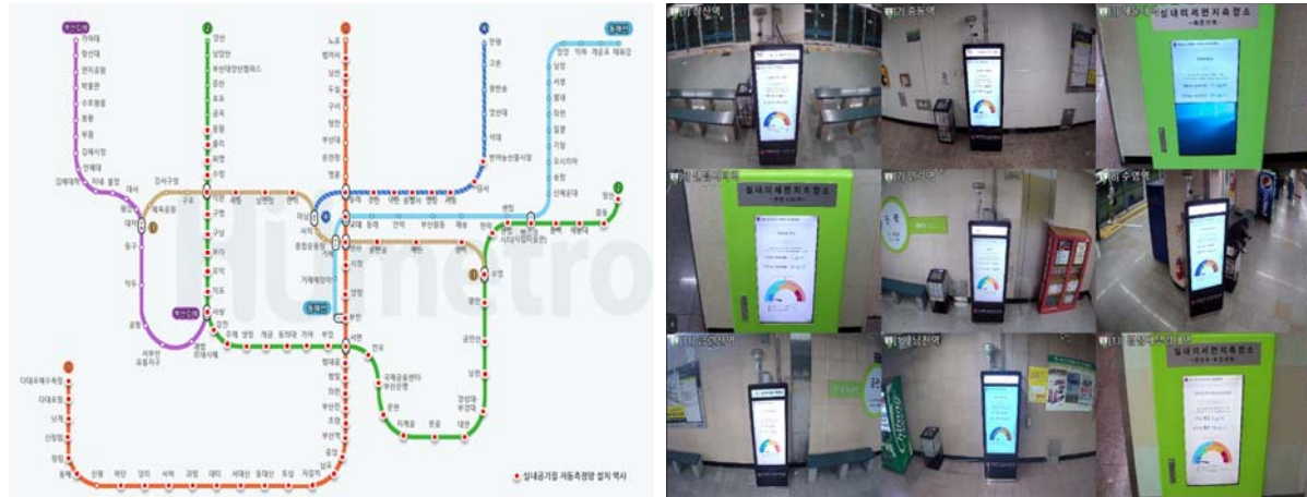
Fig. 1. Indoor air quality monitoring stations on Busan subway platforms(Red Points) and underground station indoor air quality monitoring systems.
