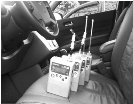
Figure 1. Scene of sampling VOCs and Aldehydes in the new car
