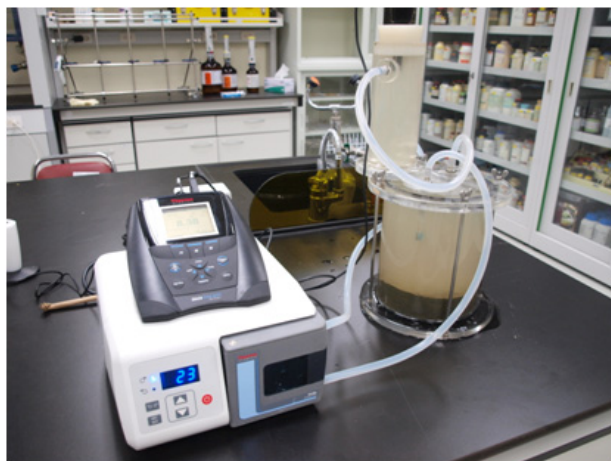
Fig. 2. Schematic of SOD measurement Apparatus.
