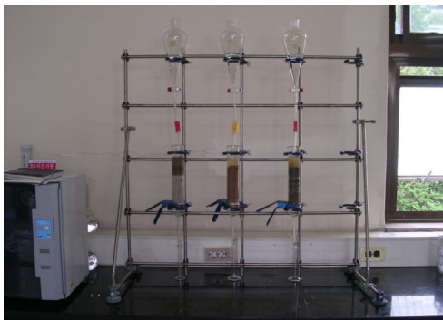
Fig. 2. Schematic diagram of column experiment.
