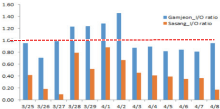
Fig. 7. PM-2.5 I/O ratio with replacement of AHU
